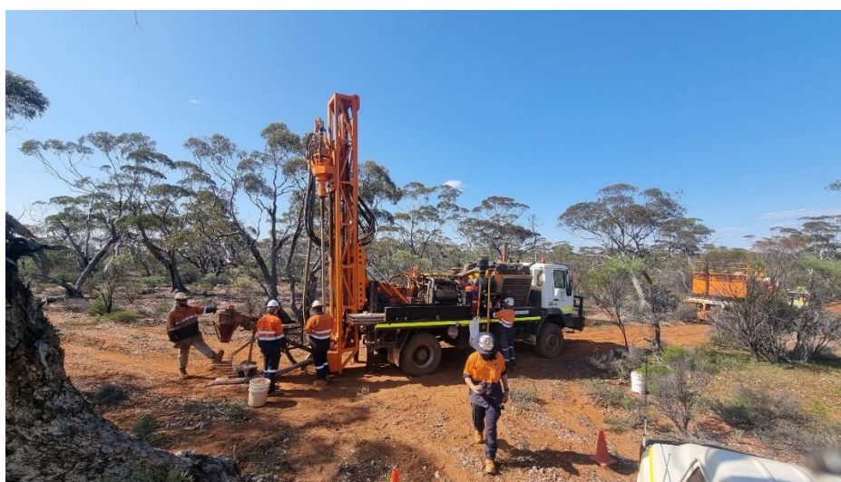
Figure 7 Aircore drill rig at Mt Jackson
