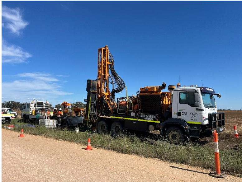
Figure 1 Drill rig commencing roadside drilling for mineral sands
